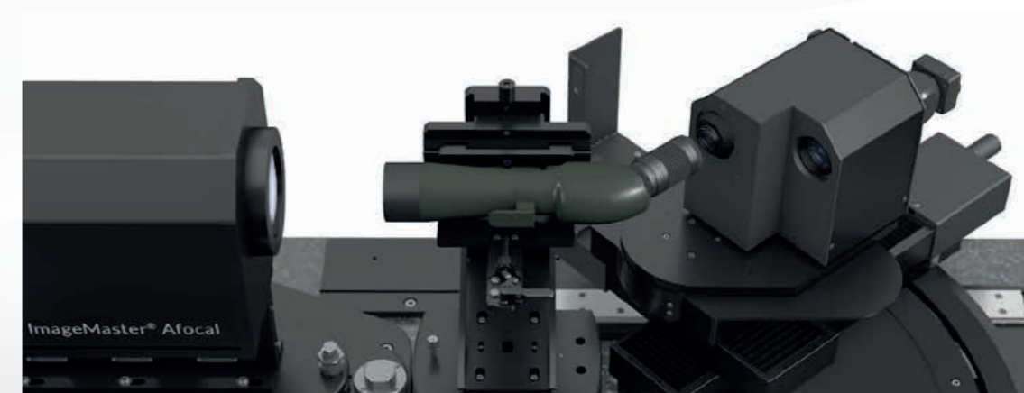
Illustration 3: Sample mounting of spotting scopes
