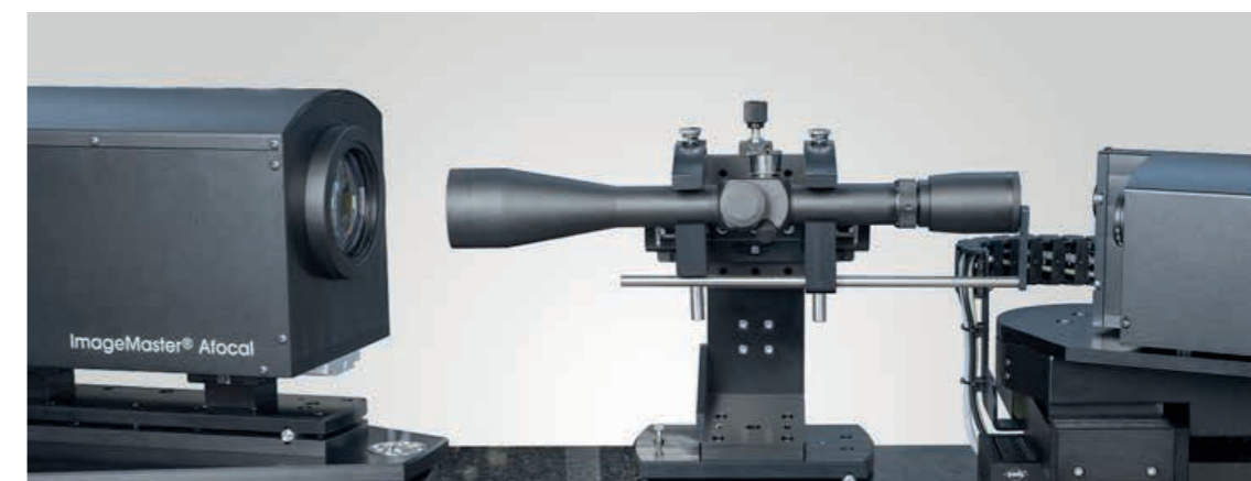
Illustration 1: Measurement of riflescopes
