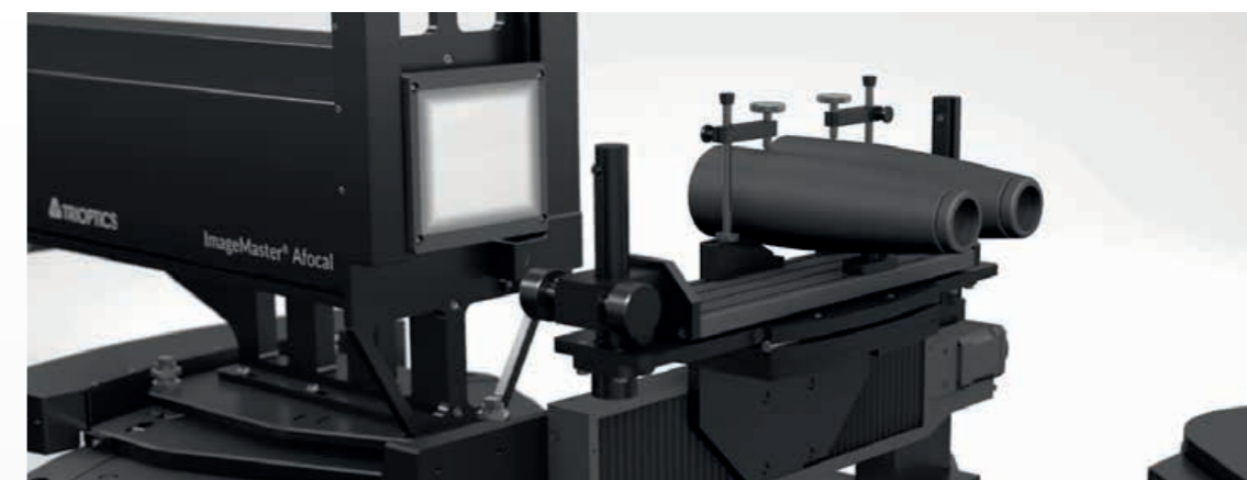
Illustration 2: Sample mounting of binoculars
